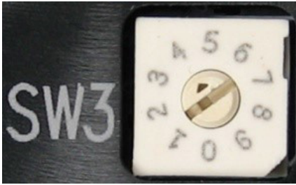
Figure 26. Ten-position rotary switch SW3.
