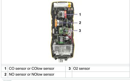
When retrofitting a sensor, the associated measurement parameter/unit must be enabled in the reading display.
