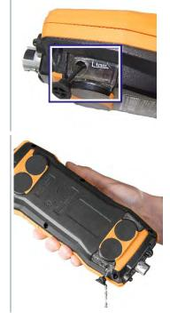
3 - Wipe off any drops still on the condensate outlet with a cloth and close the condensate outlet.
