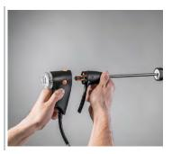
2 Fit new probe module and click into place.
